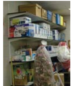
Storage of loose objects on a shelf and placement of heavy objects on top shelves should be avoided.
